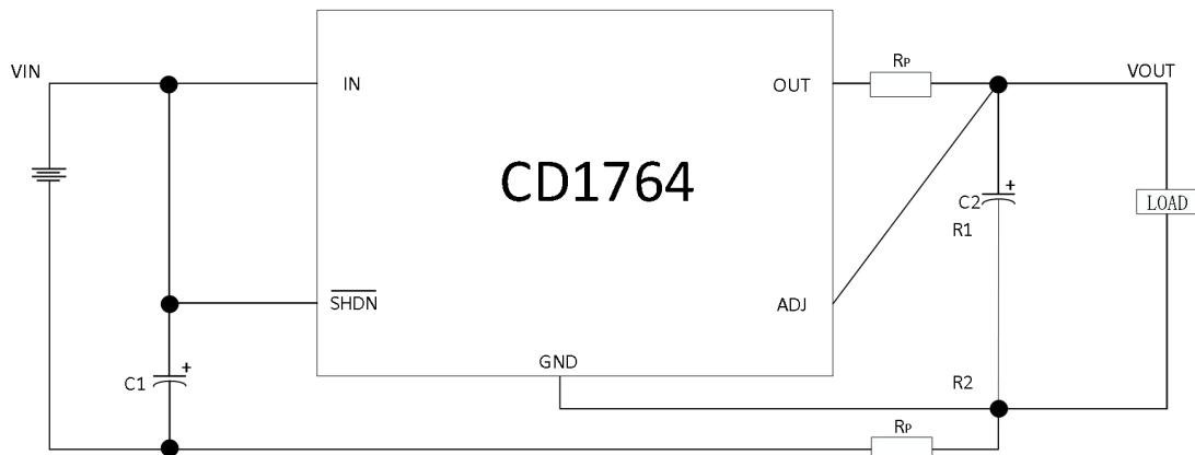
Adj (5 pins): adjustable end. The adjustable output version of the product has this port, and the adj end is directly connected to the reverse input port of the internal operational amplifier. The internal embedded voltage of this port is  $\pm 7V$ . The bias current of the port is about 3ua, and the current direction is flowing into the device. The adj terminal voltage is about 1.2V, and the output voltage adjustment range is 1.2V to 20V.
