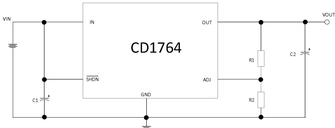
$C_1 = C_2 = 10\mu F$  TANTALUM CERAMIC OR ALUMINUM ELECTROLYTIC
